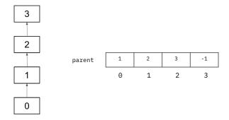
The worst case runtime of find is  $\Theta(N)$ , for find(0). Since this implementation does not use WeightQuick-Union, this could potentially arise if we unioned 0 to 1, setting 1 as the root, then unioning 1 to 2, setting 2 as the root, and finally unioning 2 to 3, setting 3 as the root (try drawing this out for yourself!). WQU solves this "spindly set" problem by ensuring that the smaller set is merged into the larger one, so when we try unioning 1 to 2, 1 must be the root and not the 2.
